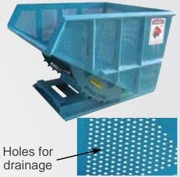
6500 LB. Capacity Heavy Duty Hopper. Open design, dewatering hoppers have perforated sides and back that allow for open drainage of wet materials. Suggested uses include: Water and Sewage treatment, paper, rags, wood pulp, recycling etc.
