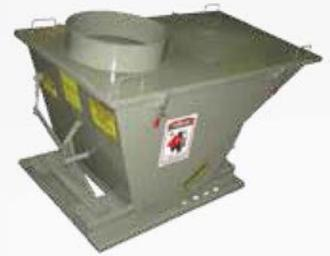
This hopper is used for the containment of dust when attached to dust collection equipment. The hopper fits under the dust collection unit and the drum collar easily connects to the hose. When full, the lid can be removed from the hopper and the hopper can be dumped using fork lift.
